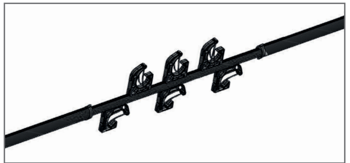
4. Option C is to position rods above and below. This configuration may provide the most compact option.
